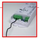
5. Repeat steps two through four for the positive wire from the power supply. The positive wire will go into the positive wiring slot.
