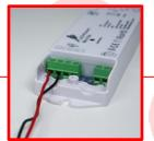
On the right side of the receiver, connect the first LED fixture. First, take the negative wire, and repeat steps two through four above, but connect the wiring in the right side green wiring block using the negative wiring slot. Repeat again for the positive wire but using the positive wiring slot.
