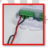
6) On the right side of the receiver, connect the LED fixture, being careful to match the correct color wires with the matching ports. The Positive wire is usually connected using the red (+) positive Terminal on the top right of the receiver.
