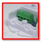
4) Take the negative wire and insert the exposed metal end into the negative wiring slot located below the screw. Place the wire inside until the wire stops against the wall inside the negative wiring slot. Take the Philips Screwdriver and turn the negative wiring screw clockwise until the screw is snug. The negative wire has now been secured to the receiver and should not come out. If it does come out, repeat from step two, and place the exposed metal wire further into the negative wiring slot.
